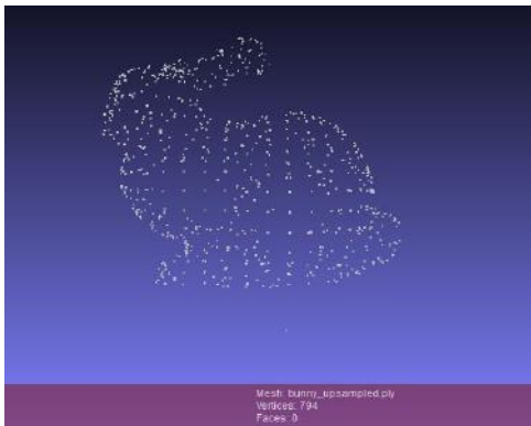
Fig. 5. Upsampling of the bunny model using proposed decision framework
