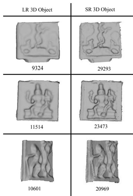
**Fig. 10.** Results for the proposed super resolution algorithm. Left column shows the 3D Objects of Low Resolution (LR) point cloud data. Right column shows the 3D Objects of Super Resolved (SR) point cloud data.
