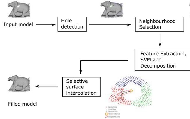
Fig. 6. Proposed hole filling algorithm.
