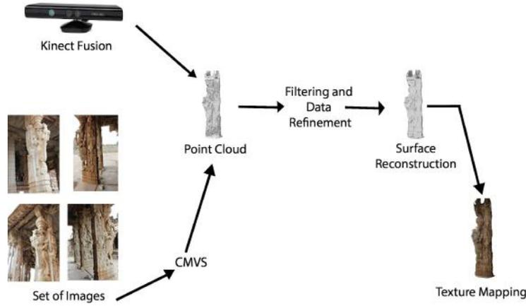
**Fig. 4.** Overview of the data acquisition and data refinement pipeline for detailed reconstruction.
