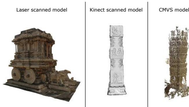
**Fig. 9.** Figure shows the 3D reconstructed models from Laser scanner for stone chariot, Kinect model for a pillar at main mantapa and CMVS model for a pillar at kalyan mantapa.
